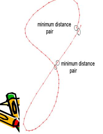
Minimum distance pair: a pair of points which has the minimum nonlocal distance in a given area.
