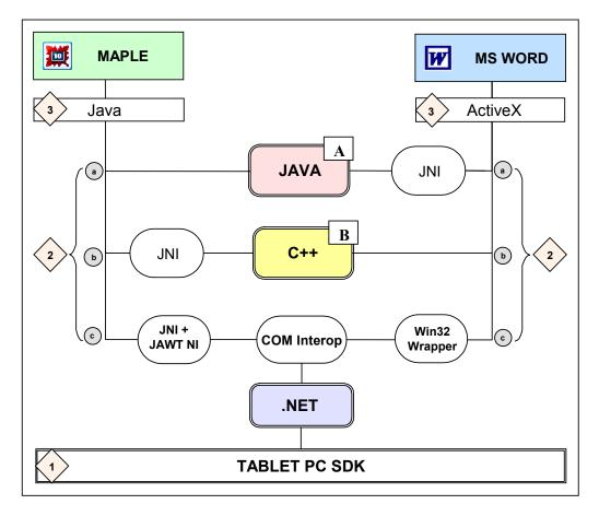
Figure 7. Implementation of the framework instantiated for Maple and MS Word applications on the Tablet PC platform
