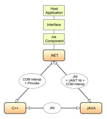
Figure 5. Linkage in the framework instantiated for Tablet PC.
