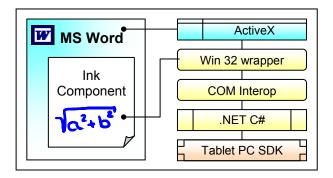
Figure 6b. Interface to MS Word: ActiveX control, accessing Tablet PC SDK ink objects
